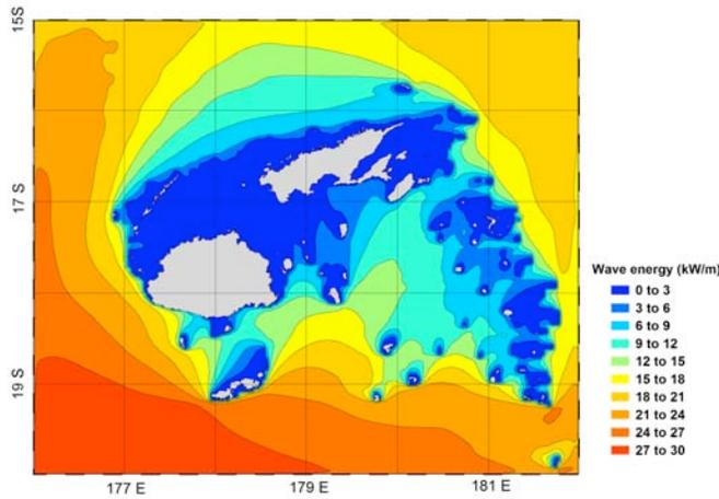
Figure 5. Fiji Islands – Wave Energy Flux (in kW/m)
