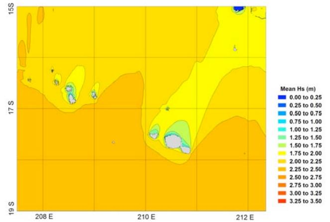
Figure 6. French Polynesia – Mean Significant Wave Height ( $H_s$ )
