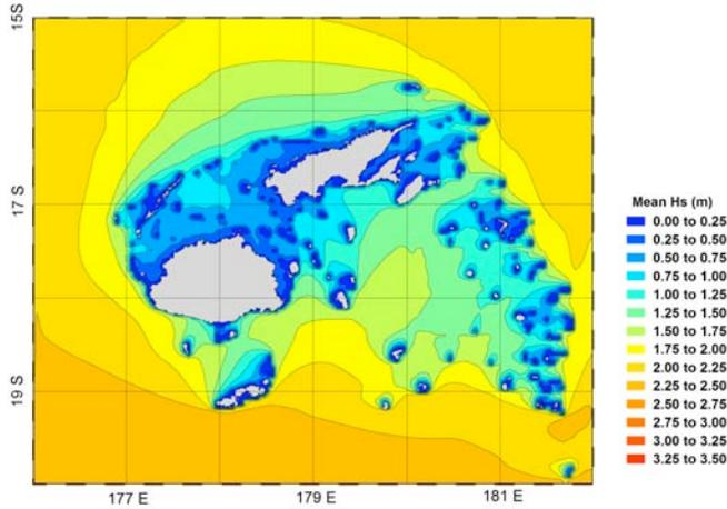
Figure 4. Fiji Islands – Mean Significant Wave Height ( $H_s$ )
